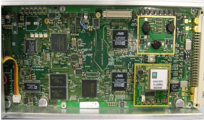
Fig. 6: The prototype RBS module board implementing the NTP synchronization algorithm. Note the OCXO in the right low corner.
