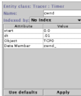
Figure 6.3: Configuration of the tracer object to record the cwnd_ field of the TCP session. This variable represents the congestion window size of the session. The tracing will start with the simulation, and will be sampled every hundredth of a second.
