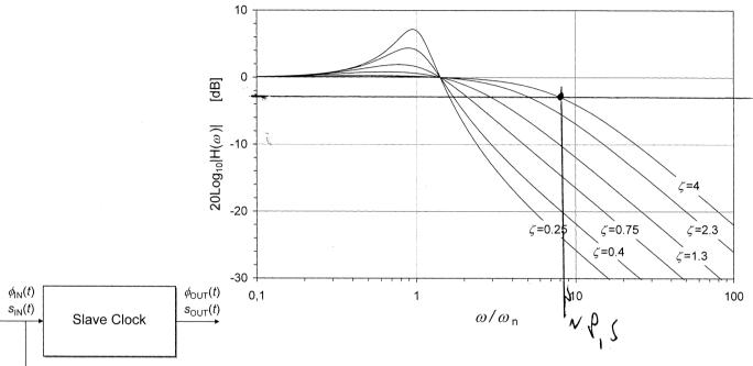
• What is the cutoff frequency (-3 dB point) [Hz] of the slave clock?
